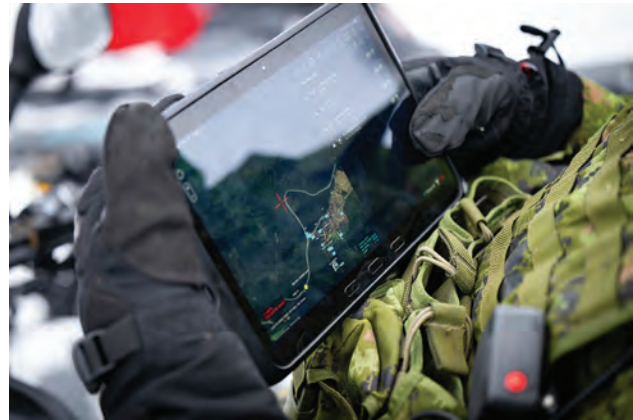
An Observer, Controller, Trainer (OCT) responsible for the evaluation of ex GLOBAL RESOLVE, tracks and updates troop movements in the training area with a Tactical Assault Kit (TAK) tablet, allowing real-time communication between different OCT elements in the field. Image taken in the Yukon Training Area near Fairbanks, Alaska, on February 17, 2026.
